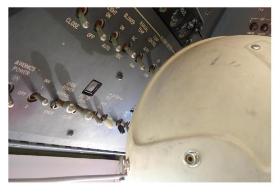
Here one can see how close the helmet is in touching the cockpit switches.
